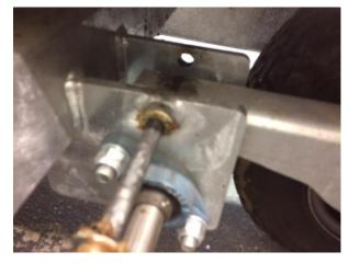
Pin removed from pivot arm ready to lower
