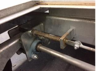
Pin locked into position above the pivot arm ready to tow.
